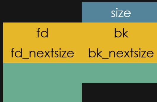
Figure 3: Inline malloc metadata
