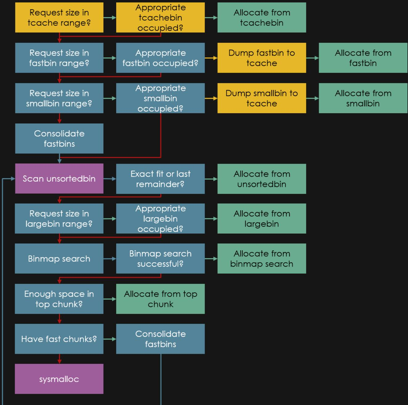
Figure 13: Malloc flowchart
