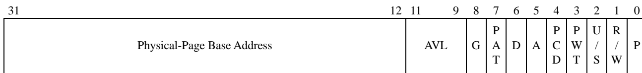
Figure 5-6. 4-Kbyte PTE—Non-PAE Paging Legacy-Mode
