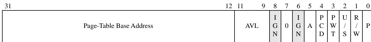
Figure 5-5. 4-Kbyte PDE—Non-PAE Paging Legacy-Mode
