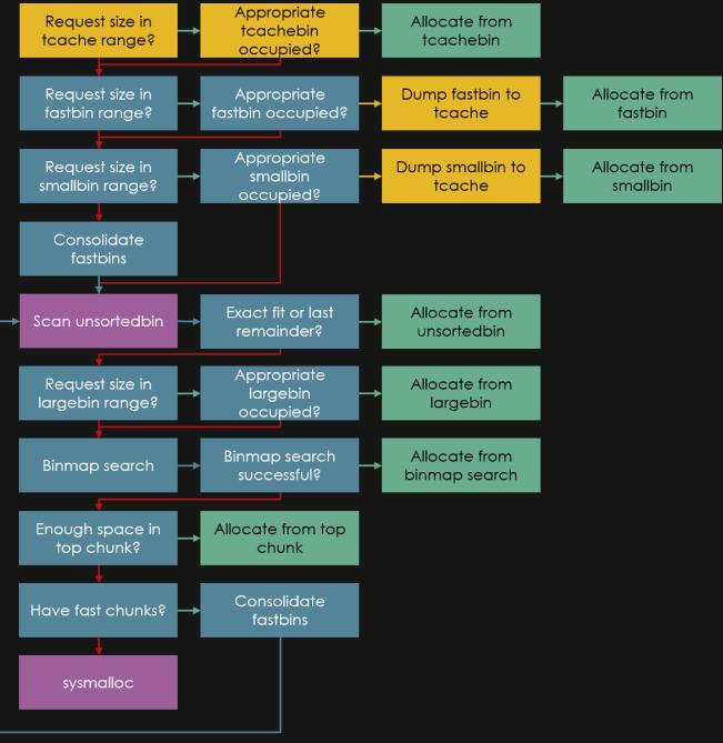
Figure 13: Malloc flowchart
