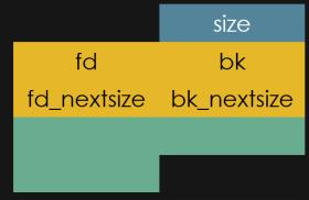
Figure 3: Inline malloc metadata
