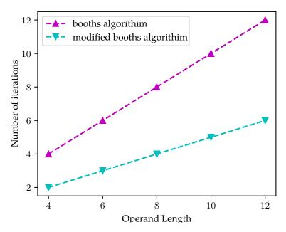
Figure 1: Add and Subtract operations of various Operand Lengths
